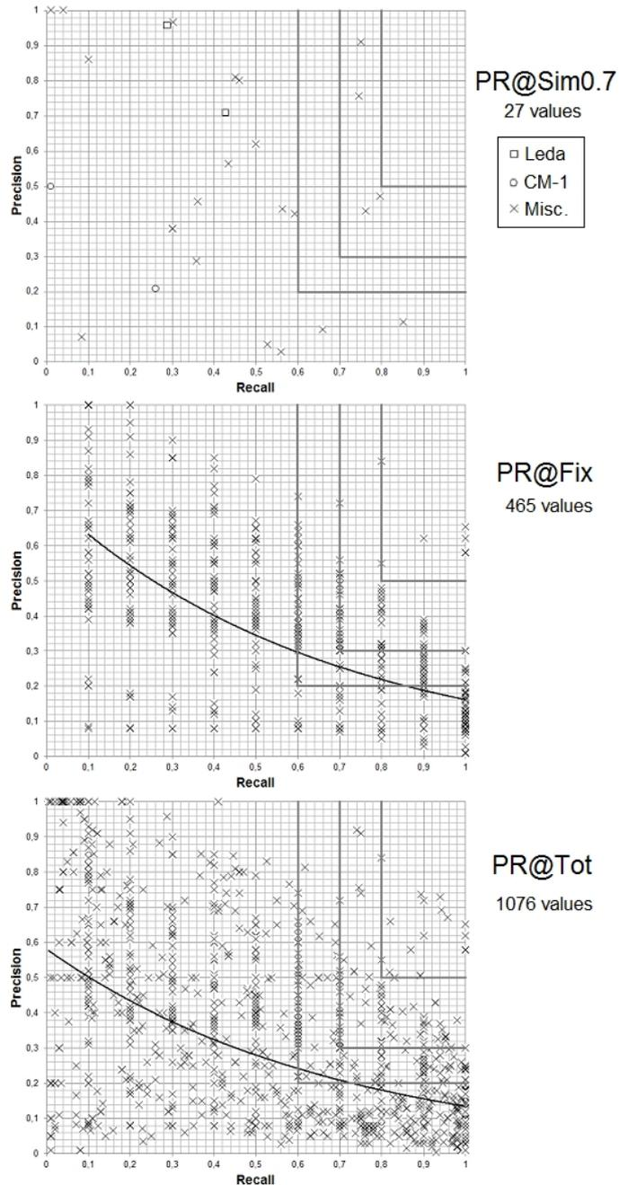
**Figure 15:** P-R footprints for trace recovery tools. The figures show P-R values representing a cut-off at the cosine similarity 0.7 (PR@Sim0.7), precision at fixed recall levels (PR@Fix), and an aggregation of all collected P-R values (PR@Tot). The figures PR@Fix and PR@Tot also present a P-R curve calculated as an exponential trendline.
