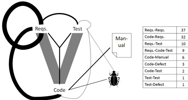
**Figure 10:** Types of links recovered in IR-based trace recovery. The table shows the number of times a specific type of link is the recovery target in the primary publications, also represented by the weight of the edges in the figure.
