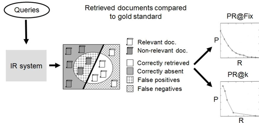
**Figure 1:** Traditional IR evaluation using P-R curves showing  $PR@Fix$  and  $PR@k$ . In the center part of the figure, displaying a document space, the relevant items are to the right of the straight line while the retrieved items are within the oval.
